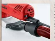
By means of the Venturi principle, the extraction channel that is integrated in the base plate ensures excellent extraction directly at the saw blade. The tracing is blown clear from one side and the chips are extracted from the opposite side. This keeps the tracing free of chips and is always easy to see even without a vacuum cleaner connected.
